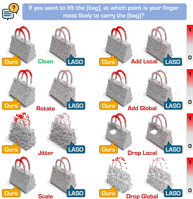
Figure 1. 3D affordance prediction under varied data noises. Given a textual prompt, previous methods like LASO [32] (right side of each example) exhibit reduced robustness across different corruption types. In contrast, our proposed method, GEAL (left side of each example), maintains high accuracy and generalization across these challenging scenarios by effectively transferring knowledge from a large-scale pre-trained 2D foundation model, enhancing robustness and adaptability under diverse conditions.
